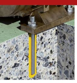
A two-component paste with a polyester resin base for the rapid realisation of structural fasteners and anchors for inserts and connectors in general. This quick-setting resin (which hardens in just 6 minutes at 20° C) facilitates the use of metal inserts a mere 2.5 hours from installation.
