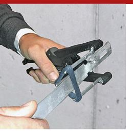
Special dilating pliers with three noses, to facilitate the installation of the rectangular seals Ringseal L19 in a central position with respect to the metal blade caisson spacers for wood formwork.
