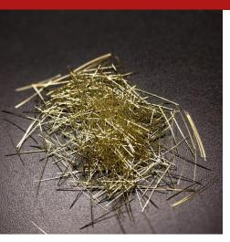
Brass-plated steel micro-fibres, obtained by cutting metal wire, for structural reinforcement of cement-based conglomerates in general. Readymesh MR is a very thin brass-plated steel wire with a diameter of 0.22 mm and a length of 6 or 20 mm, mainly used for reinforcing concrete and high-performance mortars. Readymesh MR are available in two different lengths: Readymesh MR-060 = 6 mm; Readymesh MR-200 = 20 mm
