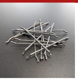
"Carbon steel fibres, obtained by the cutting of metal wire, with improved adhesion profile, for three-dimensional general structural reinforcement of cement-based conglomerates. The addition of Readymesh MF-500 significantly increases the mechanical performance of the structure in terms of toughness, ductility, fatigue, dynamic stress, shock, wear, tensile and shear strength and even post-cracking and damage behaviour."
