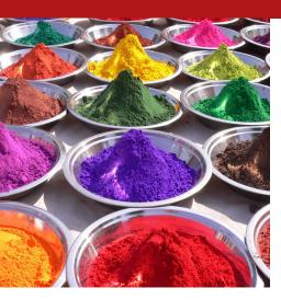
Protech Oxicrom is an inorganic oxide/hydroxide based powder compound. Added in appropriate quantities and homogeneously distributed, it is ideal for the pigmentation of cement or similar conglomerates, plaster and paint. Protech Oxicrom oxides are available in yellow, red, brown, green, blue and black.
