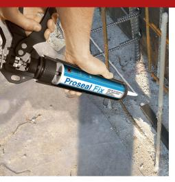
Permanently elastic, modified silane-based polymeric adhesive for sealing gaskets, joints and curbs, of both bentonitic (e.g. Clayseal 25.20, Clayseal 25.20 SW) and hydro-expansive rubber (e.g. Sealgum 20.05), for waterproofing cast elements. The adhesive is a substitute for the more traditional nailing of sealants.
