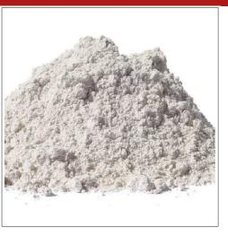
Selected white silica fume for the production of high density and high performance conglomerates (waterproofness, chemical stability, mechanical strength etc.), for packaging sulphate-resistant, anti-leaching mortars, plasters, grouts and concretes.
