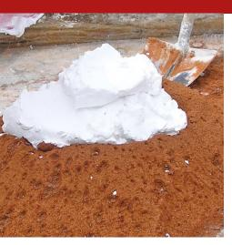
Additional compound based on ground "old" bricks and tiles, to be added to mixtures of hydraulic lime and aggregates, for producing mortars, plasters and subbase screeds, similar to the compounds of tradition "cocciopesto" (lime mortar with crushed pottery), in ecological building interventions and in the restoration of vintage buildings and monuments.
