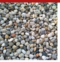
Dried, selected fine gravel, with particle size between 6 and 10 mm, specific for addition to premixed structural mortars and plasters, both castable and thixotropic, to improve or correct the particle size curve, based on the required increase in casting thickness.
