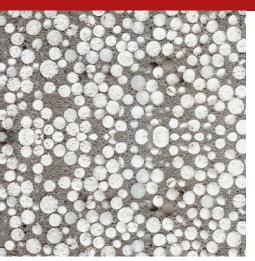
Aerating agent in solution specific for concretes exposed to freeze-thaw cycles and antifreeze salts or for light conglomerates (concrete with polystyrene, concrete with perlite, etc.). It compensates for partial lack of very fine parts in the conglomerate, improving its appearance, the cohesion and pumpability. It improves the workability, it reduces segregation and bleeding.
