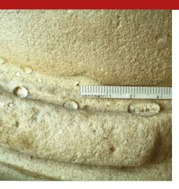
Water-repellent silicone consolidating product in aqueous dispersion, formulated for hydrophobing, anti-salt treatment and consolidation of absorbent mineral building materials, including alkaline ones. It does not cause chromatic variations or alterations in breathability. Material with very low VOC content.
