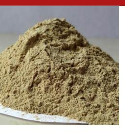
Claygrain is a dissolved, anhydrous sodium bentonite powder, characterised by a montmorillonite content in excess of 95%, with low yield-point (proof). The product should be used as it is, to increase the amount of bentonite in punctual areas, or mixed with cement and water or just water to obtain a slightly expansive waterproofing mortar, suitable for smoothing any crawl spaces in the concrete prior to laying and refilling the Claytex bentonite sheet.
