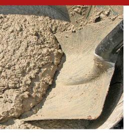
Natural hydraulic lime, hazel-coloured, obtained through firing, in a vertical oven in refractory stone and bricks, at temperatures of  $1100^{\circ}$ C, of constant quality select marly limestones, specific for mortars, plasters and substrate screeds in ecological building works and in interventions of historical and monument restoration.
