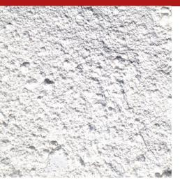
Natural hydraulic lime, white coloured, obtained through firing, in a vertical oven in refractory stone and bricks, at temperatures of 1100°C, of constant quality select marly limestones, specific for mortars, plasters and substrate screeds in ecological building works and in interventions of historical and monument restoration.
