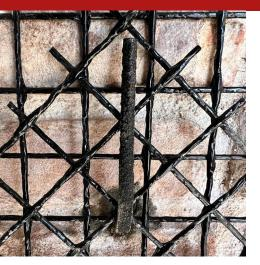
Preformed GFRP connector with improved adhesion surface, with "L" shape, 10 cm short side and long side available in different lengths, from 15 to 100 cm. Armaglass Connector L is used to mechanically connect ARMAGLASS networks to various supports (brick walls, stone walls, concrete, wood). The connector is perfectly compatible with the most common materials used for grouting, both resinous (epoxy, polyester, vinylester) and with mortars and grouts based on aerial or hydraulic binders.
